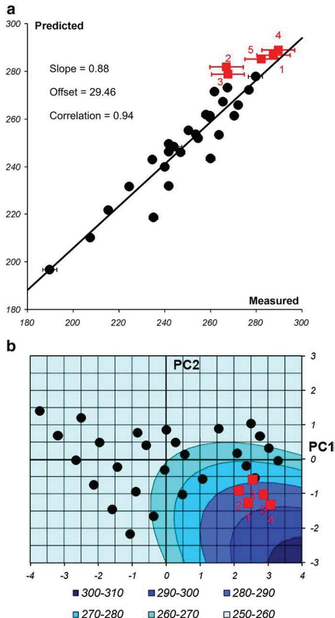
Fig. 4. Heat resistance predicted by NPCR. Dots are calibration values, squares (with error bars) are the optimized candidates. a) Predicted vs. measured plot. b) Contour map. Color intensity reflects the property value.
