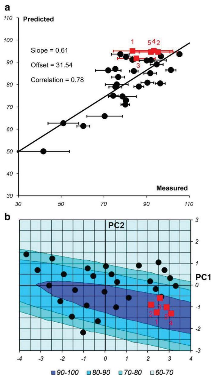
Fig. 5. Compression strength predicted by NPCR. Dots are calibration values, squares (with error bars) are the optimized candidates. a) Predicted vs. measured plot. b) Contour map. Color intensity reflects the property value.
