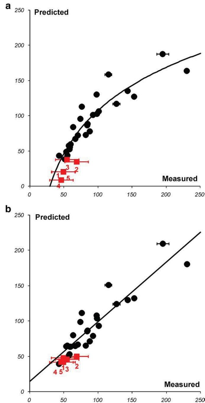
Fig. 2. Viscosity prediction. Dots are calibration values, squares with error bars are the optimized candidates. a) PCR model; b) Two-step NPCR model.
